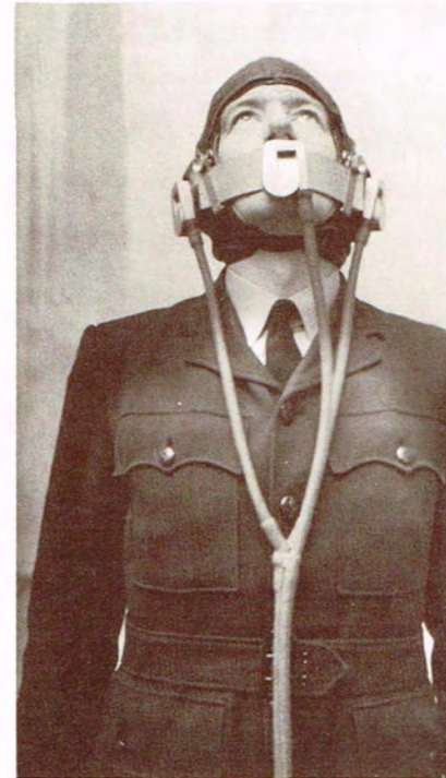
One of the first inventions of the acoustic laboratories was the Murray speaking tube, used for communication and to provide some hearing protection to air force personnel.
